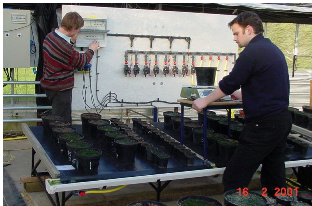
Photos 3 – 4. Year 1 experiments. Comparison of materials for capillary lift (left) and examining influence of Mypex and Tex R covers on capillary contact (right).
