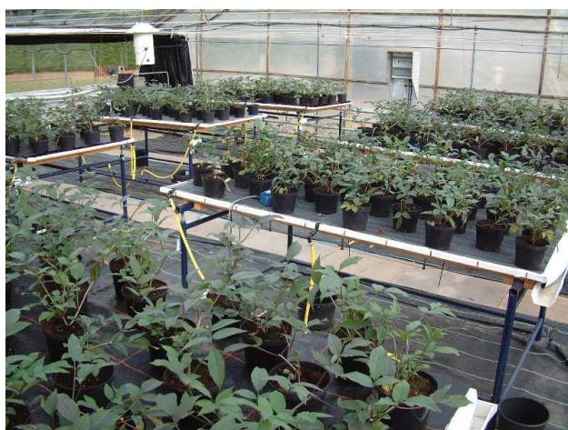
Photos 5 – 6. Small-scale beds used for testing sloped capillary flow irrigation.
